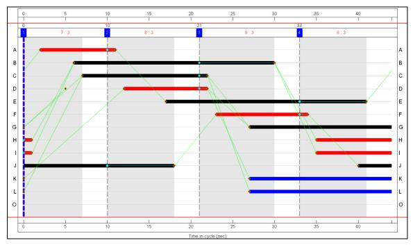
Fig. 6 – MOVA ACS stage / phase view – minimum sequence.
