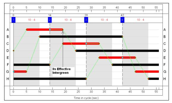
Fig. 2 – ACS Phase/Stage relationship for a 4-arm roundabout.
