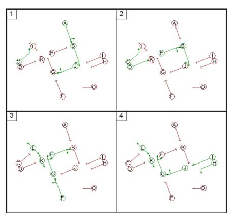
Fig. 4 – MOVA ACS coordination at a 4-arm roundabout – U-turns at red.
